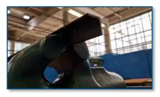
Marking the cutting plane with a file
