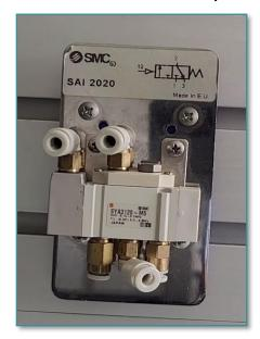
3/2 monostable valve pneumatically operated
