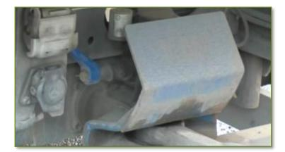
Checking that the hand grip of the tow rail is in the upper position
